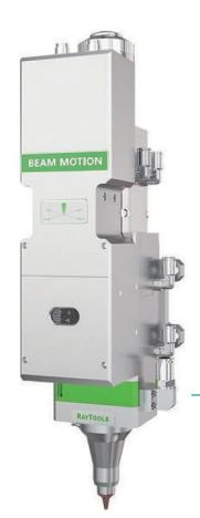
3 Cover glasses (top, middle and bottom) to protect collimation & focus lens.
